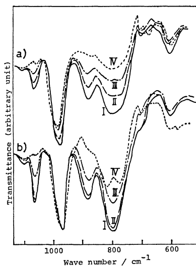
Fig. 1. IR spectra of HPA treated with ethyl methyl ketone ( 7\text{ mmHg} ) † for 30 min. a) Preevacuated at 130^\circ\text{C} for 2 h and treated at I: room temp, II: 130^\circ\text{C} , III: 178^\circ\text{C} , and IV: 240^\circ\text{C} . b) Preevacuated at room temp for 5 min and treated at I: room temp, II: 50^\circ\text{C} , III: 90^\circ\text{C} , and IV: 125^\circ\text{C} .
