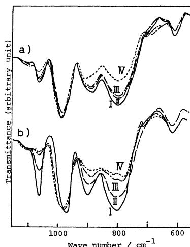
Fig. 2. IR spectra of HPA treated with 1-butene ( 7\text{ mmHg} ) for 30 min. a) Preevacuated at 130^\circ\text{C} for 2 h and treated at I: room temp, II: 122^\circ\text{C} , III: 185^\circ\text{C} , and IV: 225^\circ\text{C} . b) Preevacuated at room temp for 5 min, after which water ( 4\text{ mmHg} ) was added and treated at I: room temp, II: 124^\circ\text{C} , III: 175^\circ\text{C} , and IV: 220^\circ\text{C} .
